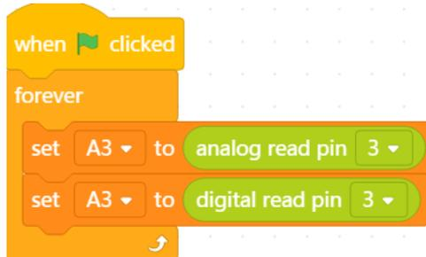
If, for example, we connect a button on pin 3 (which in principle is an analog pin), when we press it D3 will be 1 and, otherwise, it will be 0.
