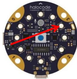
In mBlock5 LED RGB it is controlled with several specific blocks that allow to indicate a colour name or the value of each component colour (red, green and blue).
