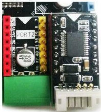
(3) Connect the terminal of DC motor (Orange) to the green contact 1A+ and 1A- on MegaPi (1B+ and 1B can be connected to the other motor).
